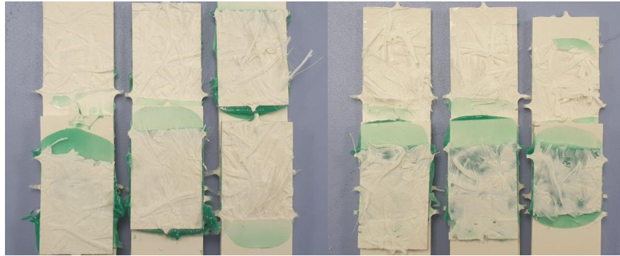
2 nd substrate applied 10 & 15 min after bead application. 1 mm bond line / water wipe / 210 sec at 83°C
